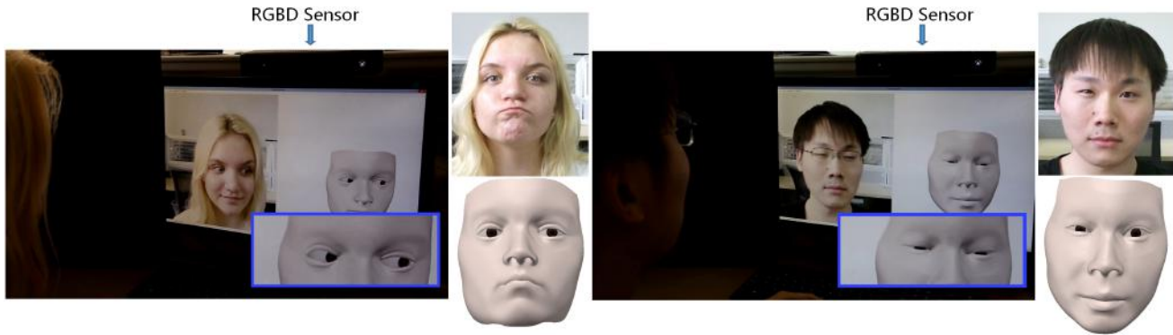
Fig. 1. We present an approach to reconstruct and track 3D eyelids in real time. This technique is integrated into a face and eyeball tracking system to obtain full face results with more detailed eye regions, again in real time (blue rectangles show closeups of the eye region). Our technique successfully reconstructs both eyelid shapes and poses, for instance the shapes of eye contours, double-folds and bulges in the center-left result and the pose differences between the two eyes in the right-most result.
